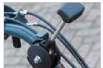
Variator - well-rounded with infinitely adjustable brush speed.
