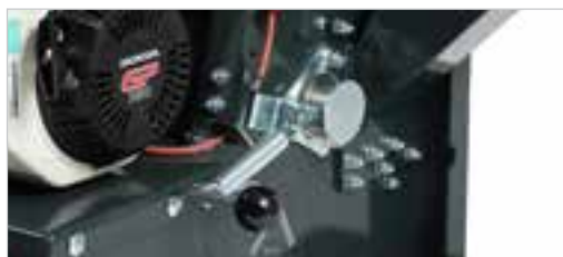
Sieve lever - for opening and closing.
