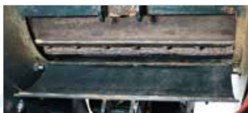
Maintenance flap – the drum housing can be cleaned of foreign bodies through the maintenance flap.
