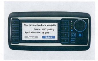
Pop up on the controller screen when spreader reaches a preset work site.
